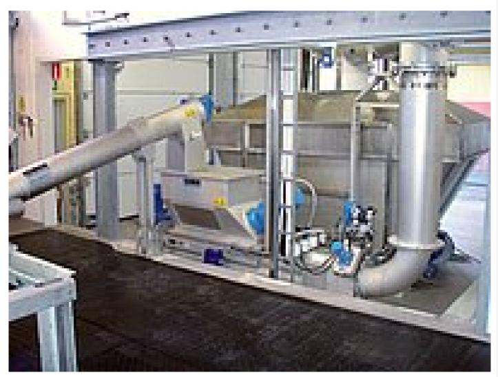
Screenings Wash Press for washout of organics and controlled high-pressure dewatering
