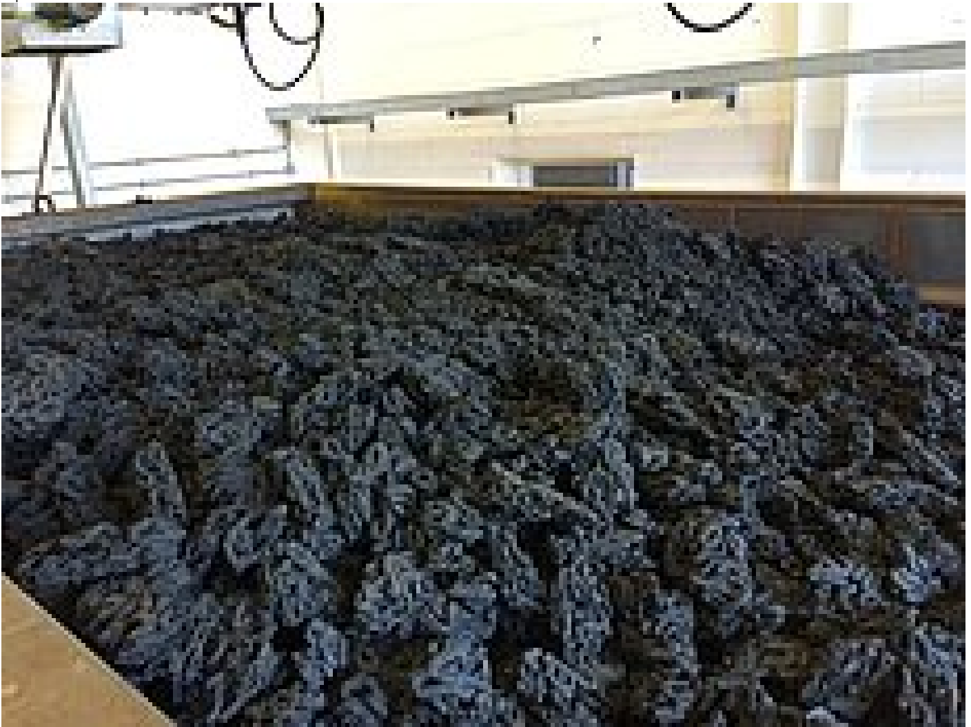
Dried sewage sludge in the transport container
