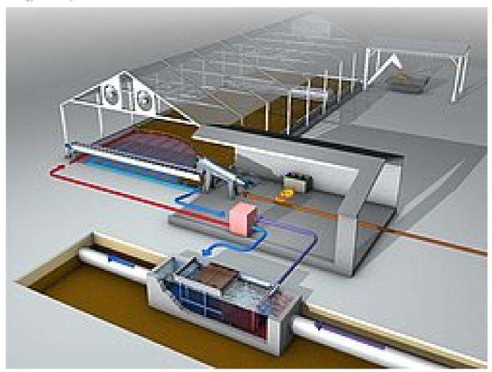
Sewage sludge disposal is a key issue on sewage treatment works. Irrespective of the way of sludge utilization, sludge weight and volume are the main causes for high costs. State-of-the-art technology offers several dewatering options but most of these solutions disregard the rich energy potential of filtrate water. The wastewater heat exchanger HUBER RoWin utilises this energy potential.
