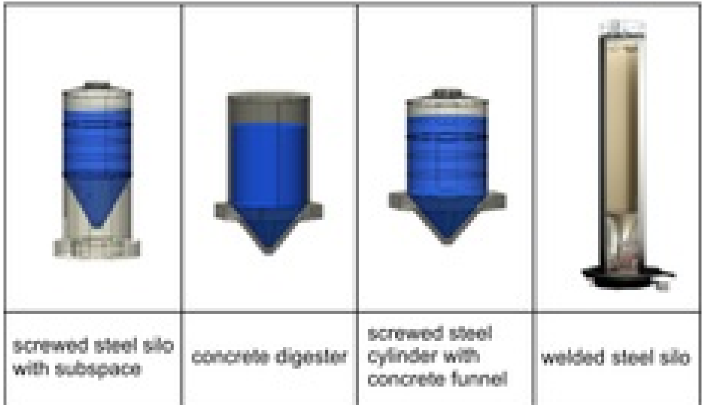
Illustration of the variants of 2-phase digestion
