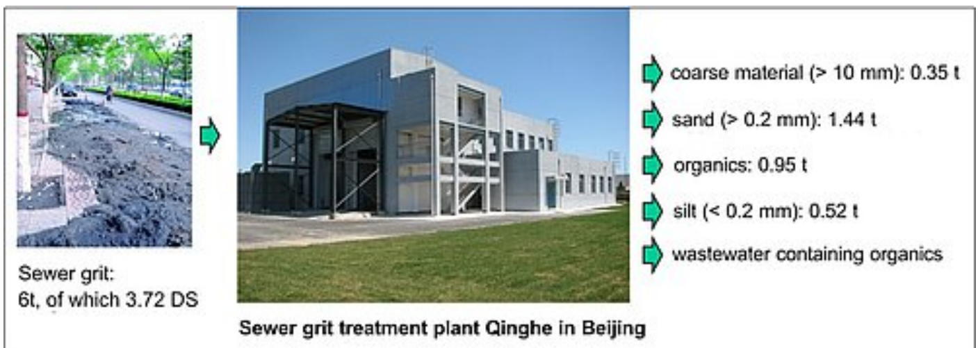
Fig 5: Material flows in the treatment plant in Beijing
