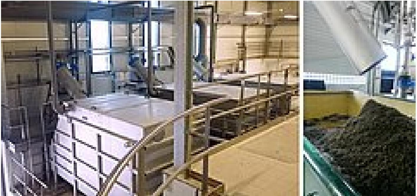
Fig. 1: Fine Screen HUBER ROTAMAT® STAR with a throughput capacity of 1.000 m<sup>3</sup>/h each providing excellent dewatering results of > 35 % DR
