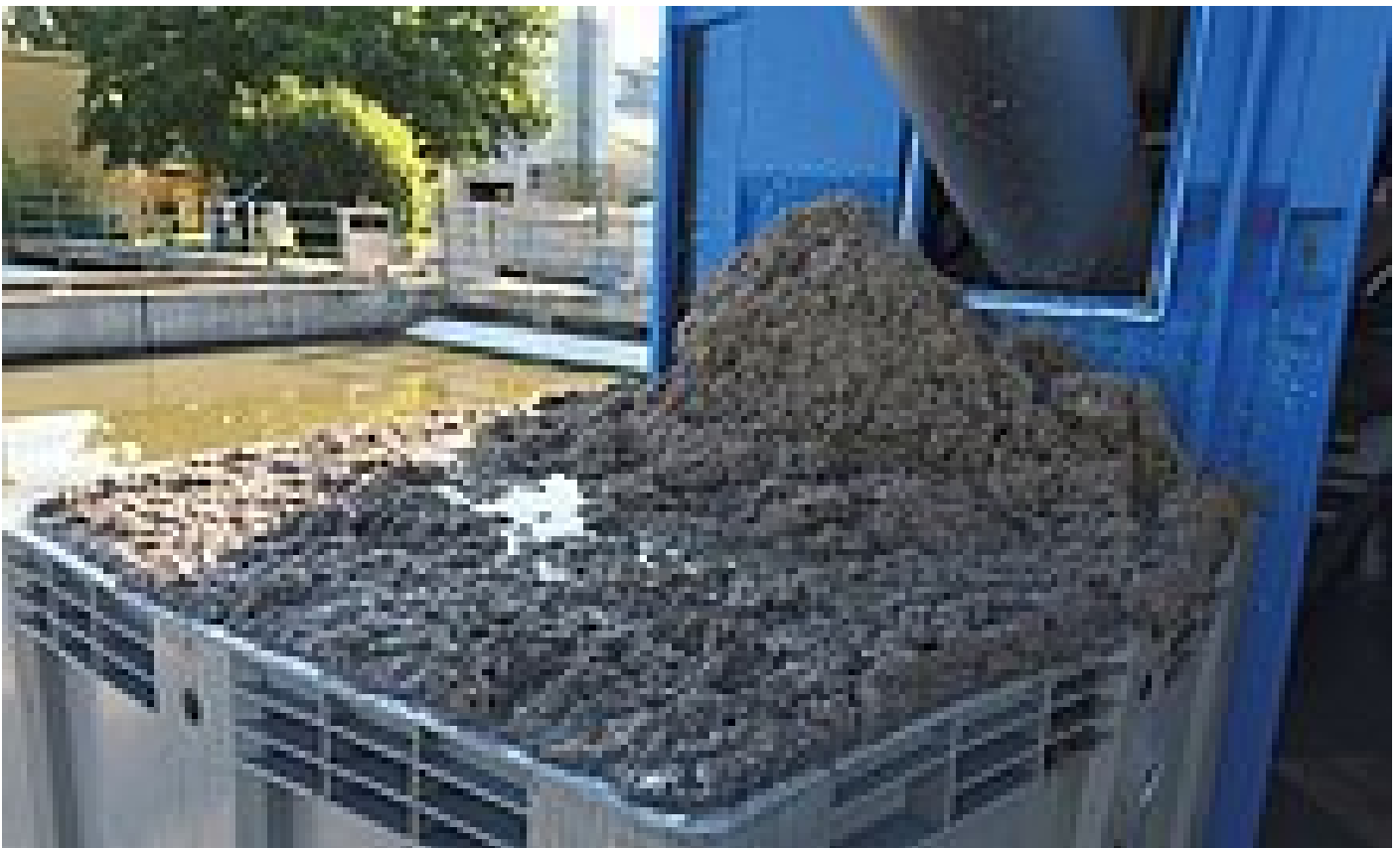
Predewatered fine screenings from HUBER Screenings Wash Press WAP® liquid for digestion
